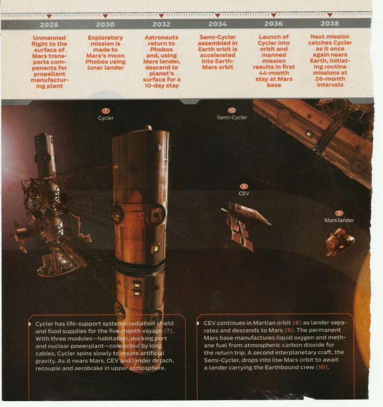
easy target for a low-propellant taxi rendezvous. Once it discharged the spacecraft to aerobrake into the Earth's atmosphere, the Semi-Cycler would be slingshot on a circuitous 14-month route back to Mars for another run.
