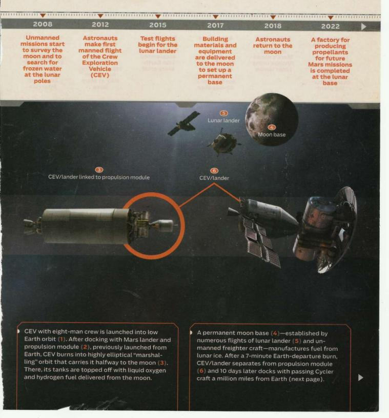
A downside of the gravity-assisted Cycler concept, however, is that the vehicle flies by Mars at quite a high speed, up to 27,000 mph. This velocity is not a showstopper on the outbound leg, where the CEV taxi craft would aerobrake, relying on the friction of the Martian atmosphere to slow down without using any propellant. But departing Mars for the leg back to Earth, the craft would need a large amount of propellant to catch up with the speeding Cycler.
